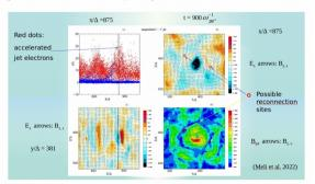
For an e'- it plasma jet: Panel a: The ix - vvx phase-space distribution of jet (red) and ambient (blue) electrons. Panels b. c. & d: structures generated due to different MI modes. Panels b & c: possible magnetic reconnection sites.
